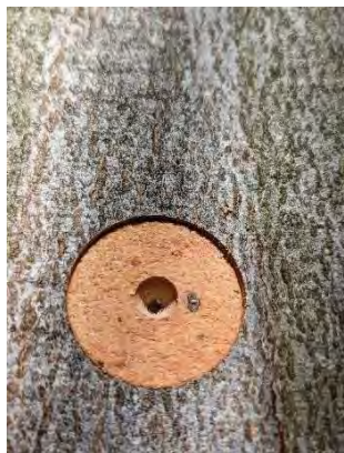
2.6.1 Create a flat surface using the 40mm diameter positioner drill bit
