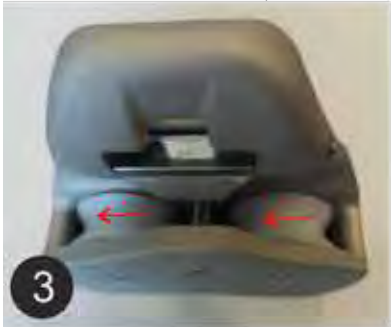
Checking of MCD wear ( Free space between Locking Part and Plate 7,5 < x < 9,3\text{mm} )
