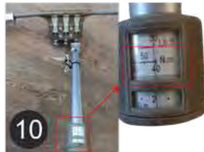
Checking the tightness of the M10 screws in CBS Anchors (= 40 N*m).
