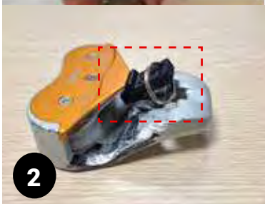
Checking of MCD wear ( Free space between Locking Part and Plate 7,5 < x < 9,3\text{mm} )
