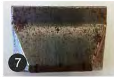
Corrosion check on MCD components.
