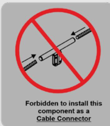
Forbidden to install this component as a Cable Connector
