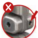
Missing little screw
