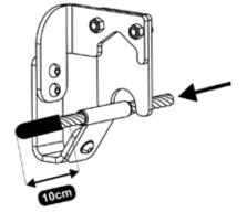
In situations where the safety cable has a large curve, the Positioners is used to provide stability to the trajectory.
