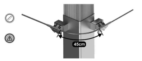
It must be ensured that the cable curve is separated from the structural element (pole or other game elements), at least 15 cm, to avoid possible MCD collisions.
