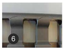
Check that IMN & CLiC-IT CBS anchorages have not suffered deformations due to shocks, deformations due to overstress in the screw housings or in the hole where the safety cable passes.
