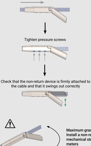
Maximum gradient: 45° Install a non-return with mechanical stop every 2
