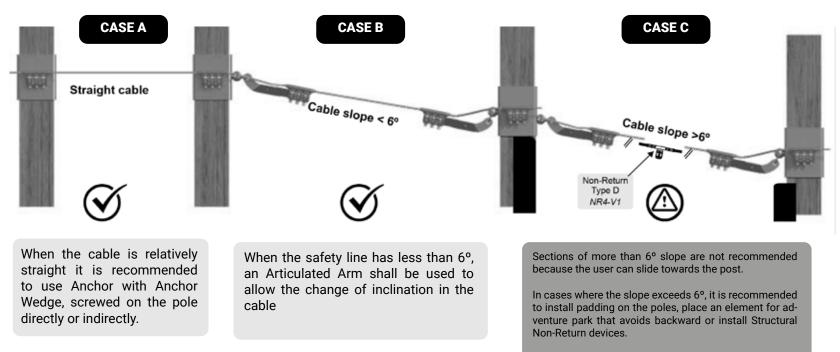
This section must be installed with Articulated Arms.
