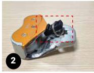
**Checking of MCD wear** (*Free space between Locking Part and Plate 7,5 < x < 8,7mm*)
