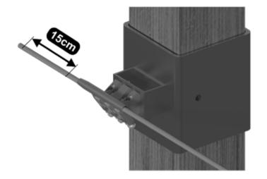
At the safety line terminals, both at the beginning and at the end, we must leave at least 15 cm of free cable that leaves in excess of the Anchor cylinder. At these two endpoints, one additional Anchor must be installed.
