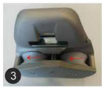
Checking the correct operation of MCD wheels
