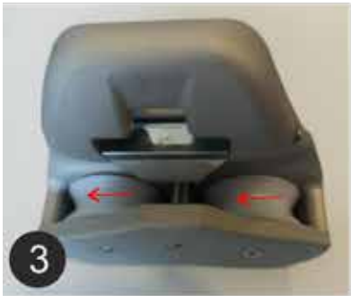
3 Checking the correct operation of MCD wheels
