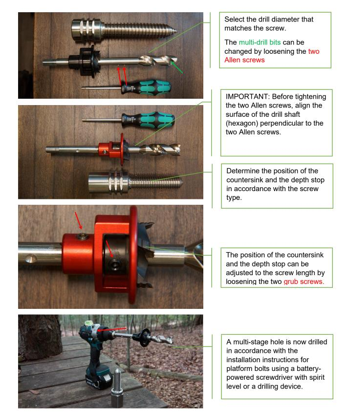
Drill-driver recommendation: use a recommended drilling torque of 800Nm (maximum 1000Nm). Caution: if the machine is too powerful or the torque is not respected, the drill bit and accessories may break.
